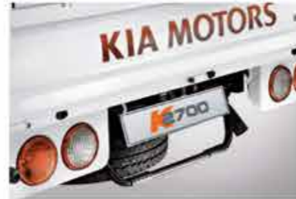
Rear license plate holder & step: Provides a convenient way to extend your reach when loading or unloading items.
