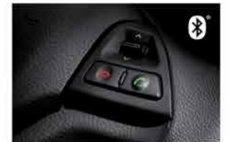
Bluetooth steering wheel controls: Enables use of your Bluetooth-enabled mobile phone for a safe journey.
